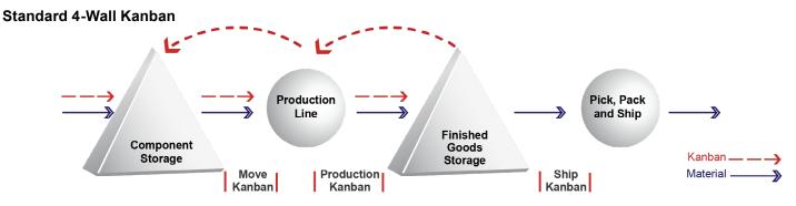
The graphic illustrates the monitoring of material flow within the plant. Electronic Kanban automatically initiates an inventory 'pull' when material replenishment is needed - thus making for a clean, efficient and effective process.
