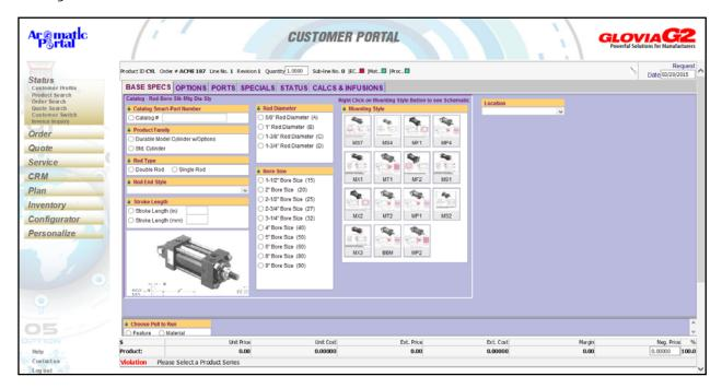
Every selection made by the user allows or removes other choices. The selection of a 1-3/8" Rod Diameter here has restricted choice of Bore Size – unavailable options are greyed out.
